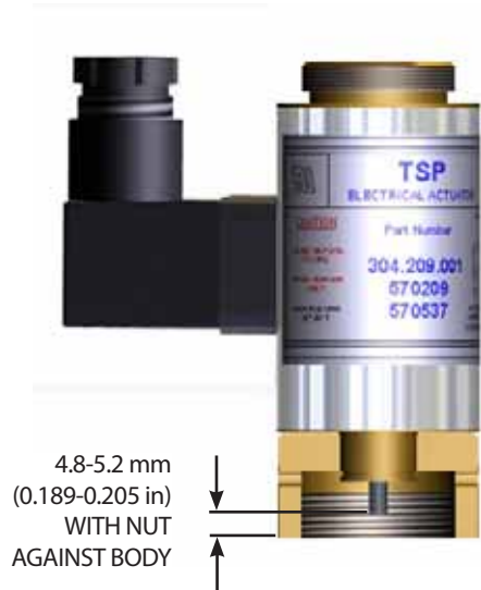
Figure 54 - Actuator Non-Fire Position
